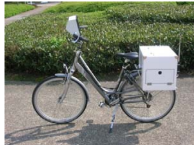
Air Quality Bike (Aeroflex) for Mobile AQ Measurements by VITO, Belgium
