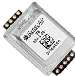
NDIR Gas Sensors (CO 2 ) by SenseAir, Sweden
